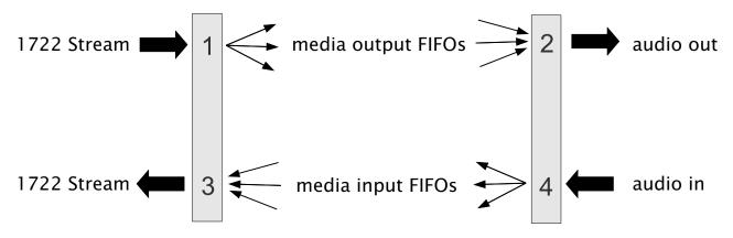
As described in the previous section, an IEEE 1722 audio stream may consist of many channels. These channels need to be routed to particular audio I/Os on the endpoint. To achieve maximum flexibility the XMOS design uses intermediate audio buffering to route audio.
